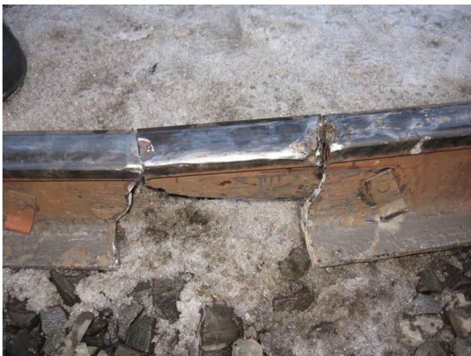
Figure 3-11: Rail Defect – Detail Fracture from Shell
