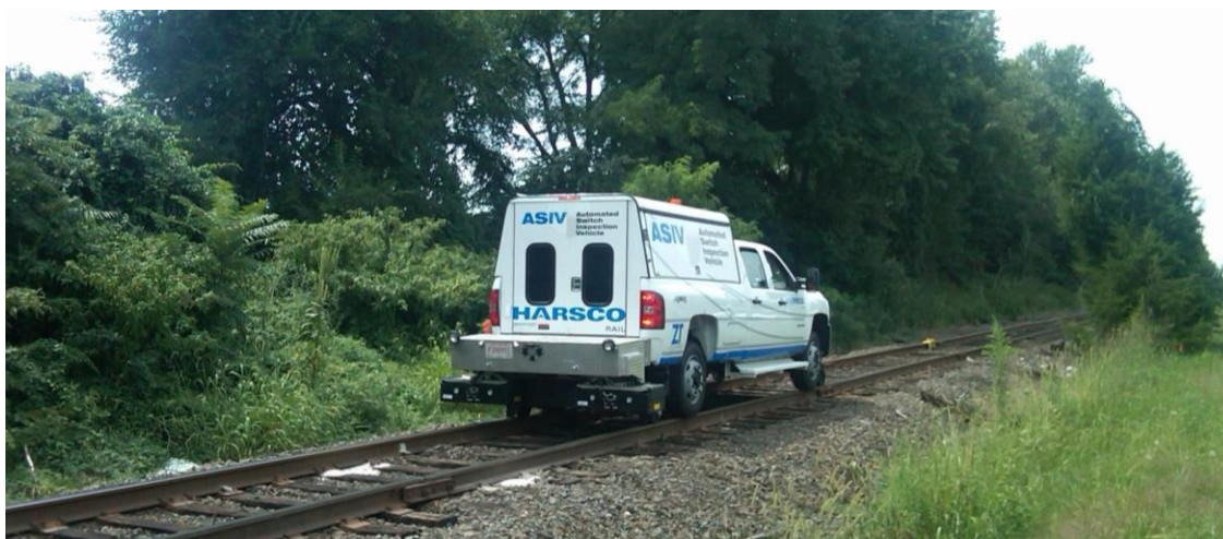
Figure 6-4: Automated Switch Inspection vehicle
