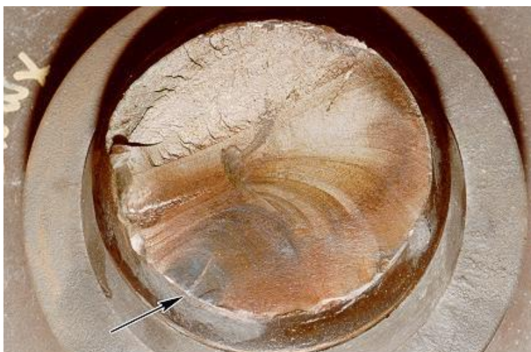
Figure 3-3: Failure surface of axle
