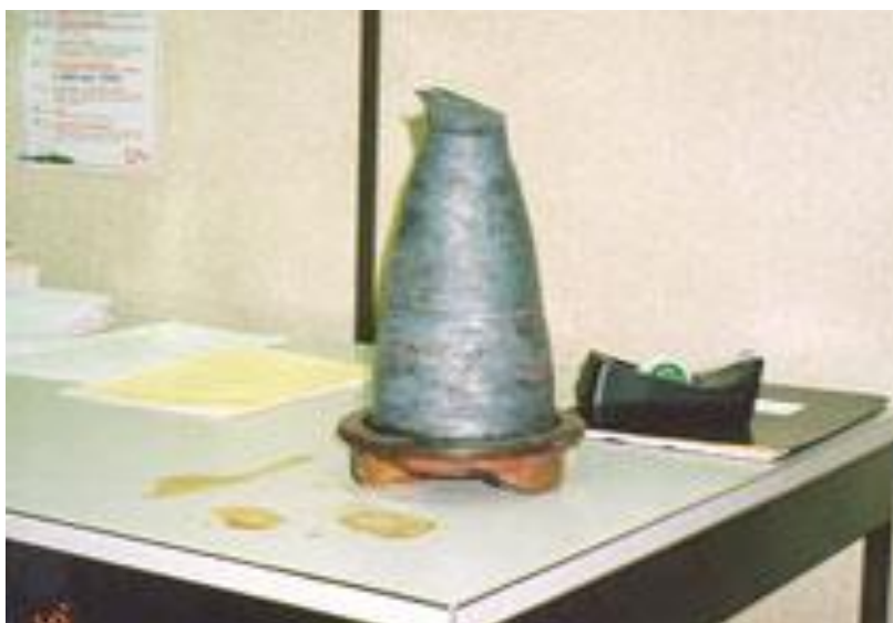
Figure 3-5: Bearing Cap with Burnt Off and Fractured Axle
