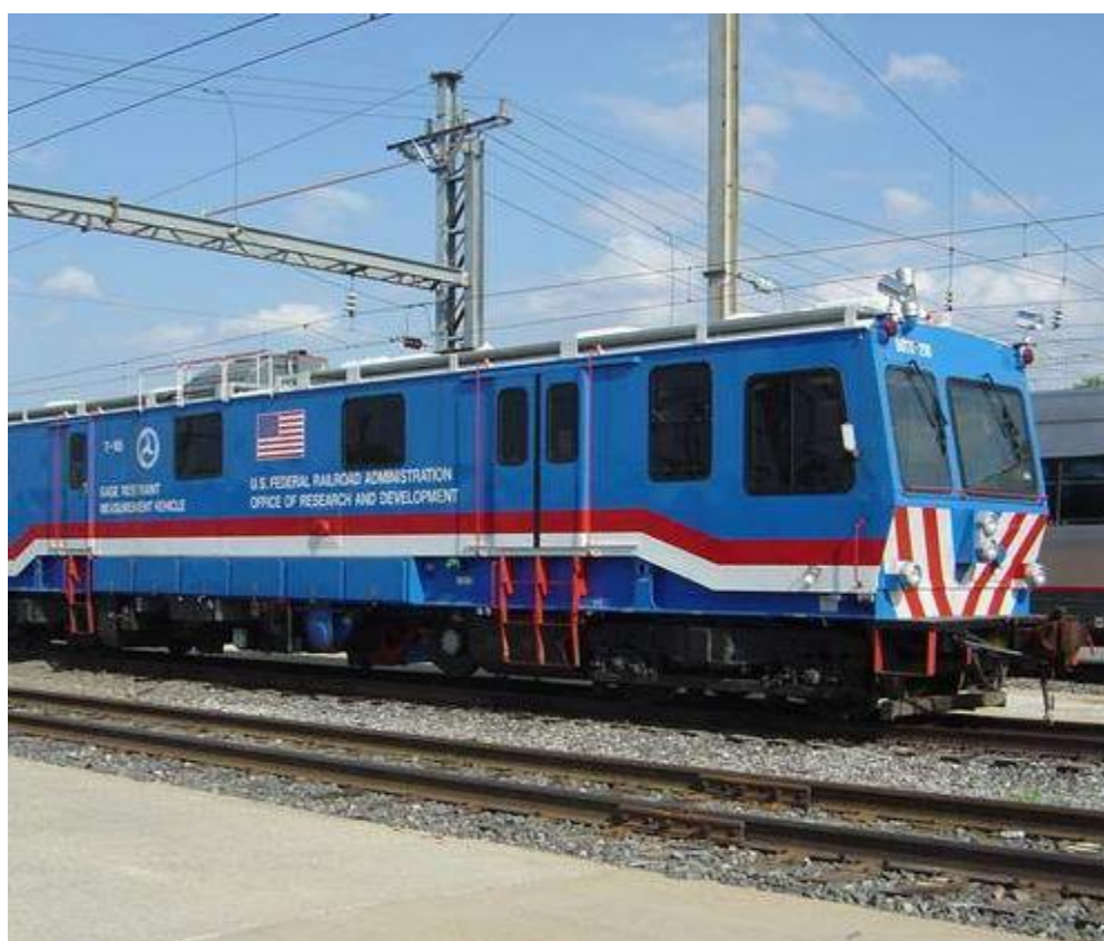
Figure 6-8: US FRA Track Recording Car with Supplemental Inspection Systems (to include GRMS)
